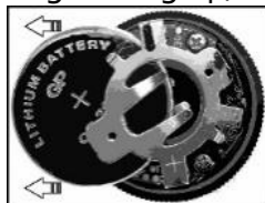
Removing the battery from the connector sleeve
